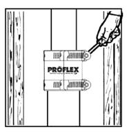
Tighten clamps to 60 inch-lbs. or torque.
